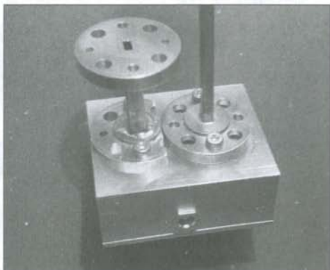
Fig. 8: Mixer version 2 with LO port and RF port
