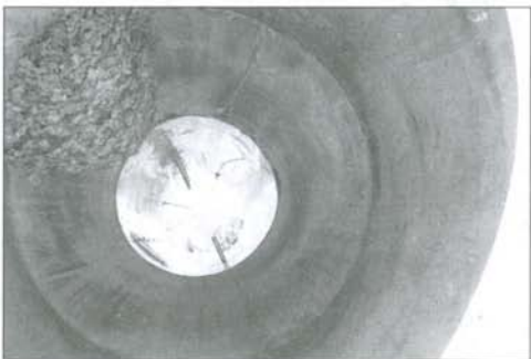
VK3UM's 23cm W2IMU feed with 2.2dB swallow nest attenuator inside
